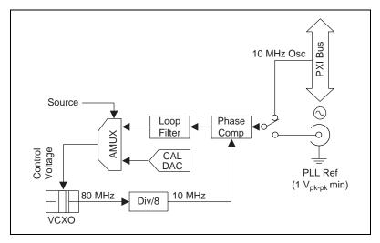
Figure 2-12. PLL Architecture for the NI 5401 for PXI
